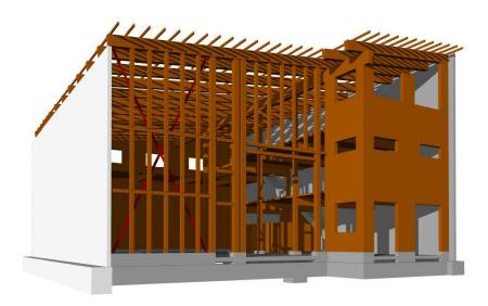
The actual installation process of CLT and Glulam is extremely efficient and straightforward. Engineered wood products are a lightweight material choice compared to concrete panels and masonry construction, resulting in simplified installation and minimal slab and footing requirements. Sophisticated manufacturing processes make a high level of prefabrication possible.
