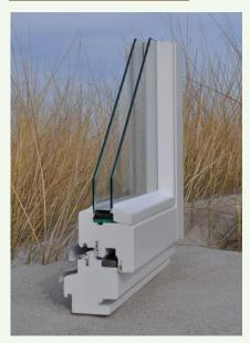
Standard U<sub>f</sub> 1.3 W/m<sup>2</sup>K Improved U<sub>f</sub> 1.1 W/m<sup>2</sup>K Standard Double Glazing U<sub>g</sub> 1.1 W/m<sup>2</sup>K TGI Spacer Glass Thickness Up to 32 mm Double Seal System
