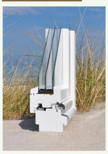
Standard  $U_f$  0.9 W/m<sup>2</sup>K Improved  $U_f$  0.8 W/m<sup>2</sup>K Standard Triple Glazing  $U_g$  0.5 W/m<sup>2</sup>K TGI Spacer Glass Thickness Up to 52 mm Double Seal System
