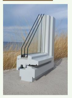
Standard  $U_f$  1.0 W/m²K Improved  $U_f$  0.9 W/m²K Standard Triple Glazing  $U_g$  0.7 W/m²K TGI Spacer Glass Thickness Up to 42 mm Double Seal System
