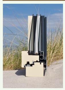
Standard U<sub>f</sub> 1.1 W/m<sup>2</sup>K Improved U<sub>f</sub> 0.8 W/m<sup>2</sup>K Standard Triple Glazing U<sub>g</sub> 0.7 W/m<sup>2</sup>K TGI Spacer Glass Thickness Up to 42 mm Double Seal System
